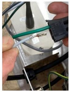
Insert black lead into remaining socket on side of connector.
