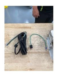
Insert white and black leads through port in side of chassis. (IMPORTANT: DO THIS BEFORE INSERTING LEADS INTO CONNECTOR)
