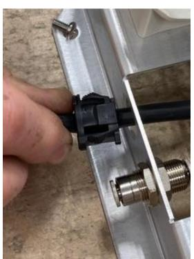
• Insert white lead into middle socket in connector until you feel it lock as shown.
